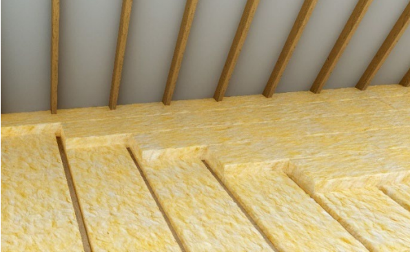
Diagram 1 - Typical installation of IndiBreathe Flex fitted between the timber joists and laid in layers on top, perpendicular to the timber joists
